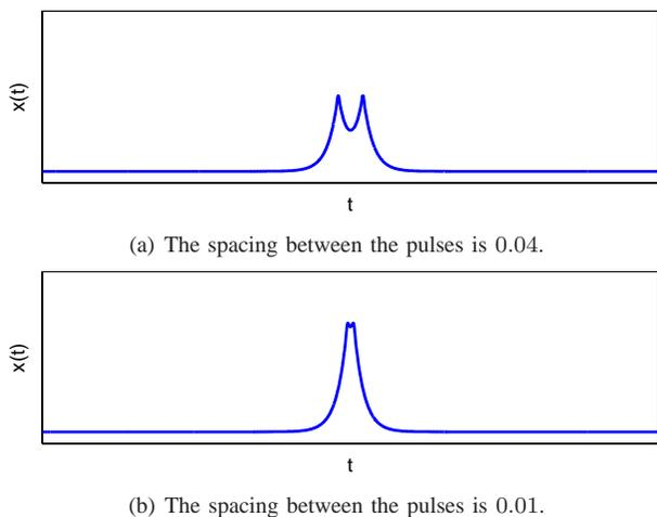
Fig. 4. Demonstration of the different levels of overlap between pulses.
